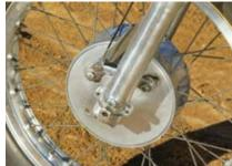
The bike is fit with a single-shoe drum front brake, but Rayborn reportedly rarely used it. He much preferred to scrub off speed by plowing the front wheel.
