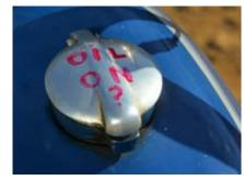
In addition to the fuel petcock, the feed line from the remote oil tank also has to be turned on before starting the bike.
