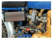
The 36mm Amal GP1 carburetor is capped with a modern K&N air filter element; Otherwise, the bike is exactly as Rayborn raced it. Even the tires are original.
