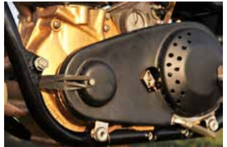
This bike is fit with countless one-off pieces built by Mann himself, like this custom fiberglass primary cover that was created to comply with another of the ad-hoc AMA rulings Mann was often subjected to.
