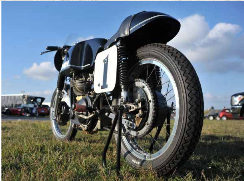
This bike is fit with countless one-off pieces built by Mann himself, like this custom fiberglass primary cover that was created to comply with another of the ad-hoc AMA rulings Mann was often subjected to.
